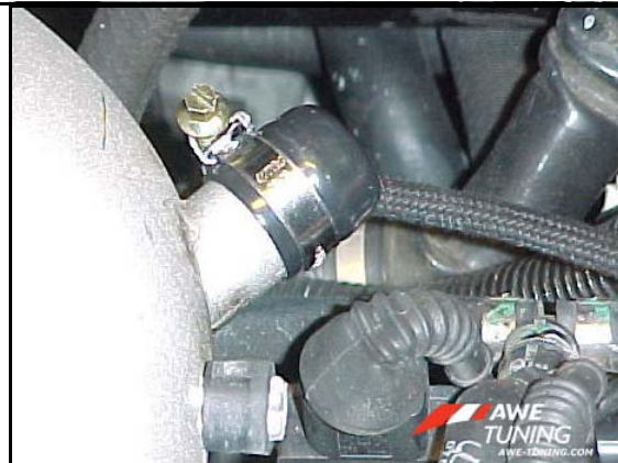
Figure 3: Capping off PCV branch
