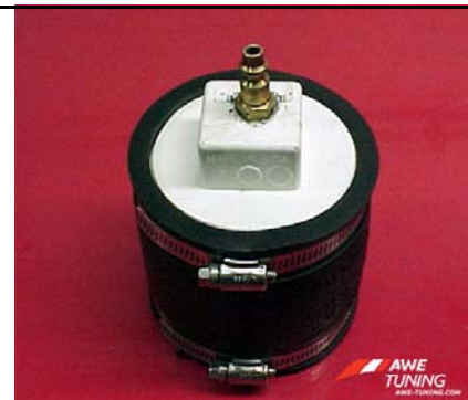
Figure 1: Fitting installed in PVC cap
